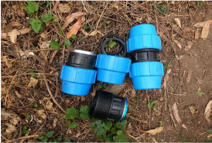
Some fittings the community procured for repairs on Karerema GFS
